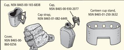
The 2-qt collapsible canteen, NSN 8465-01-118-8173, is larger and flexible. The canteen's cover. NSN 8465-00-927-7485, also has an outer pocket for water purification tablets. You can carry this canteen over your shoulder with a strap. It can also attach to your equipment belt or loadcarrying equipment. It collapses when drained for less bulk.
