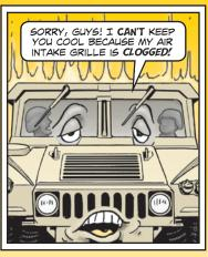
Operators, fans on your M997A3, M1151A1, M1152A1, M1165A1, and M1167 HMMWVs need to pull in a lot of air to keep you cool. But if the protective air intake grille gets clogged, that air flow is cut back dramatically. The fans can overwork and burn out.
