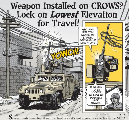
Several units have found out the hard way it's not a good idea to leave the M153 common remotely operated weapons station (CROWS) II locked at maximum elevation for travel.
